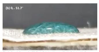
Fig. 2. Sample Image of A Silk/Resin Relationship: (a) a Phobic Relationship Between INR Epoxy and MoOH Silk, And (B) A Philic Relationship between Hydrex Vinylester and MeOH Silk.
