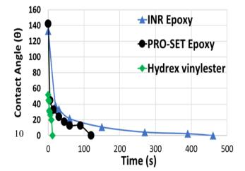
Fig. 4. Effect of Resin on the Contact Angle Change over Time for the three resin systems investigated: INR Epoxy, PRO-SET Epoxy and Hydrex Vinylester.
