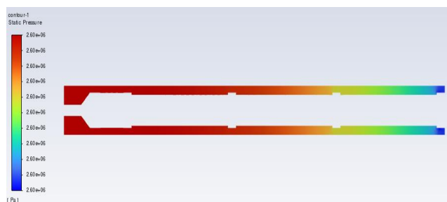
Figure 12: Single pipe pressure.
